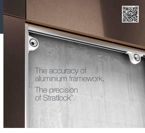
Panel mounting onto aluminium framework has never been faster or more flexible. The all-new Stratlock system uses a two-stage clip mechanism to provide 4mm of panel adjustment in any direction before locking accurately into position. The result; flexible yet exact alignment with non-sequential panel removal and acoustic isolation.
