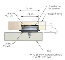
Through section showing surface mounted adhesive installation
