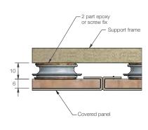
INSTALLATION: Partially exploded through section showing typical installation method
