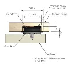
Through section showing surface mounted adhesive installation
