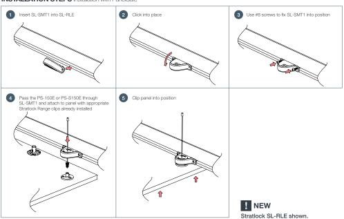
SL-SMT1 Stratlock® Sidemount - Suspension of SL-RLE with M10 threaded rod hanger
